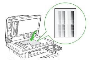
Place the test print face down on the platen glass, with the black bands along the top left edge of the platen glass. Stack approximately 20 sheets of blank paper on top of the test print for a more precise gradation correction.
