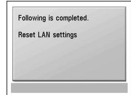
The machine's network settings are restored to factory defaults.
