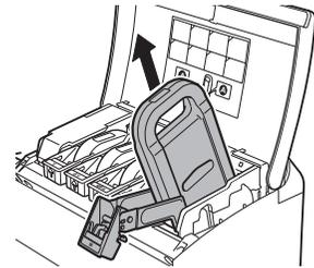
**Caution** • Store the Ink Tank you removed in the box with the ink holes (a) facing up. Otherwise, ink may leak and cause stains.
