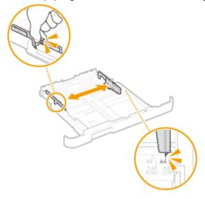
While pressing the lock release lever, move the front side paper guide to align the projection to the appropriate paper size marking.
