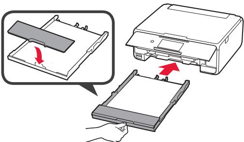
The following figure shows the state after the cassette is inserted.
