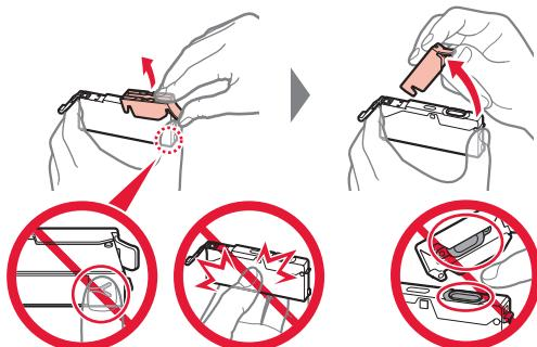
Do not push the both sides of the ink tank with the Y-shape air hole blocked.
