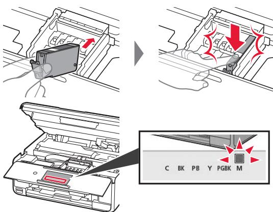
If the color is not displayed on the screen even though you have installed the ink tank, the color of the ink tank may be wrong or you may have installed an ink tank, such as one with a different model number, that is not supported by this printer. Either install an ink tank for the correct color or use the provided ink tank for setup.
