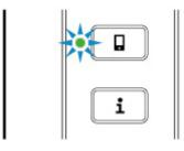
If not, press the **Direct** button once to enable Wireless Direct.
