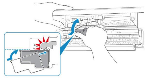
After confirming that the FINE cartridge is installed properly, close the cover.
