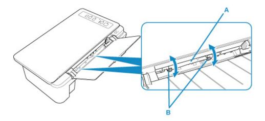
After cleaning the paper feed rollers, turn on the power, then clean the paper feed rollers again.
