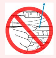
If you soil or scratch this part by touching it with paper or your hand, it could damage the printer.
