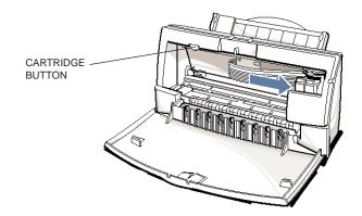
Close the printer's front cover. O Use both hands to lift the cover into place and press firmly to close it.
