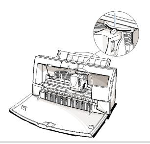
button once and close the front cover. • The cartridge holder moves to the home position on the right.
