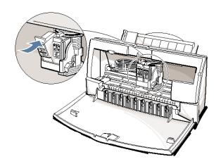
Make sure each BJ tank is correctly seated in its respective slot.
