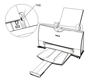
O Make sure there are no gaps between the stack of paper and the paper guide nor the right edge of the sheet feeder.
