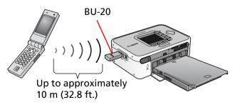
A screen similar to the following will appear in the printer's LCD monitor while data is being transmitted. The Bluetooth Unit BU-20 will also blink blue. Do not break the Bluetooth connection until transmission is complete. If the connection is broken, turn the printer off and then on again before reinitiating printing.
