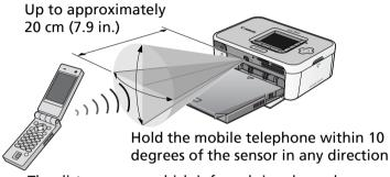
The distance over which infrared signals can be transmitted and received varies according to the mobile telephone model and operating system.
