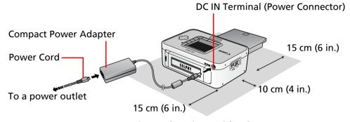
Situate the printer with at least 15 cm (6 in.) of free space in front and back and at least 10 cm (4 in.) of free space on the sides.
