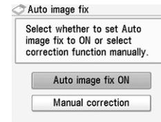
When **Auto image fix ON** is selected, the scene or person's face of a shot photo is recognized and the most suitable correction for each photo is made automatically. It makes a darkened face by backlight brighter to print. It also analyzes a scene such as scenery, night scene, person, etc. and corrects each scene with the most suitable color, brightness, or contrasts automatically to print.
