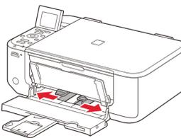
2 Slide the right Paper Guide to the end. The left Paper Guide moves simultaneously with the right guide.
