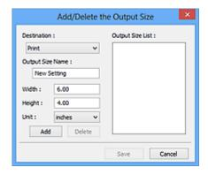
In the **Add/Delete the Output Size** dialog box, you can specify multiple output sizes and save them at one time. Saved items will be registered to the **Output Size** list and can be selected, along with the predefined items.
