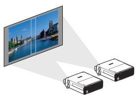
Blend the overlapping edges of images from multiple projectors to make the overall image more seamless. (P163)
