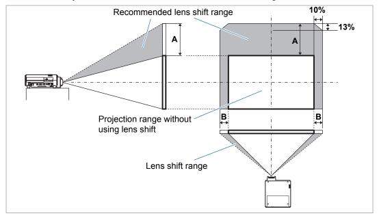
Maximum upward (A) and horizontal (B) movement using lens shift (reference values, [cm (in)])
