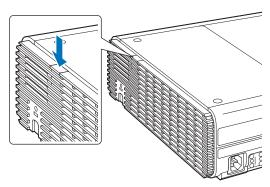
3 As you hold down the lamp cover release button, slide the lamp cover toward the back, and then lift the cover to open it.
