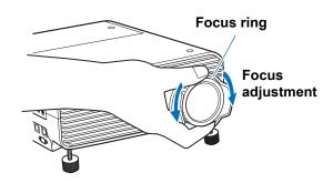
Images will waver as you turn the focus ring. Hold the focus ring on top and bottom and turn it slowly as you adjust the focus.
