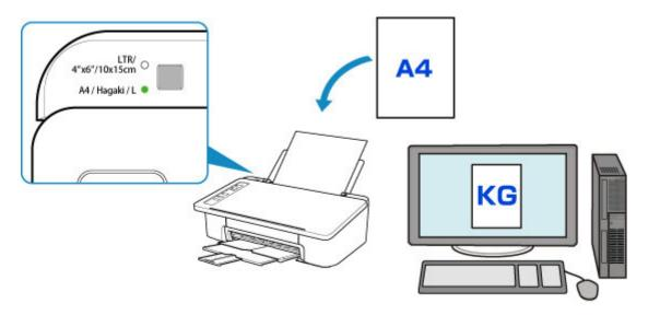
When you start printing, the **Alarm** lamp and the **Paper** lamp indicating the paper size setting for printing flashes in synchronization.
