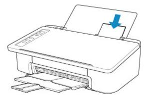
After loading paper on the rear tray, either of the **Paper** lamp lights up according to the paper size loaded last.
