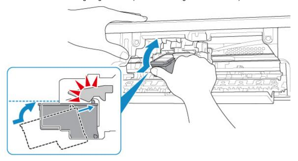
After confirming that the FINE cartridge is installed properly, close the cover.
