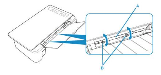
After cleaning the paper feed rollers, turn on the power, then clean the paper feed rollers again.
