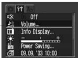
Menu items followed by an ellipsis (...) can only be selected after pressing the **SET/FUNC.** button or the ▶ button to display the next menu. Press the **SET/FUNC.** button again to confirm the setting.
