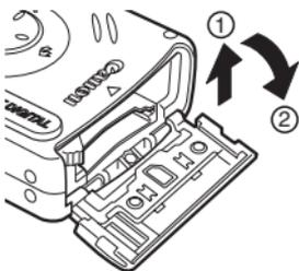
**1** Slide the SD card slot/battery cover in the direction of the arrows.
