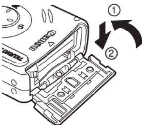
**3** Slide the SD card slot/battery cover closed.
