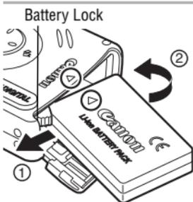
**2** Press the battery lock while inserting the battery pack all the way in until the lock clicks.
