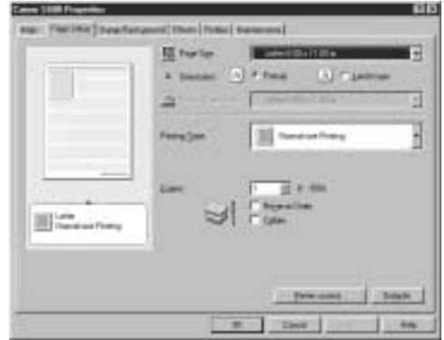
**Scaled Printing** With this option you can set the scale of the printed image down to 20% or up to 400% of the original.
