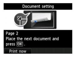
Remove the first sheet of original from the platen glass and load the second sheet on the platen glass, then press the **OK** button.
