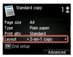
Press the right Function button to specify the orientation and the advanced layout.
