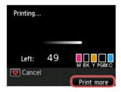
1. Press the right **Function** button when the print progress screen is displayed.
