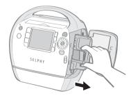
Make sure that the cartridge is oriented as shown by the direction indicator on the inside of the printer, and insert the cartridge until it clicks into place.
