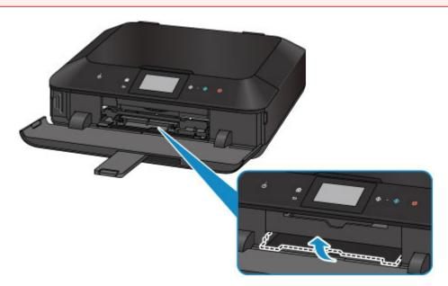
**3.** Remove the printable disc from the disc tray.
