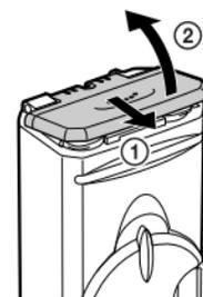
**3** Push the battery cover lock in the direction of the arrows while opening the battery cover.
