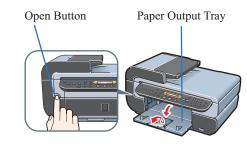
**6** Open the Scanning Unit (Printer Cover) until it locks into place. The Print Head Holder moves to the center.
