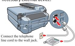
You can connect an external device (telephone or answering machine) if necessary.
