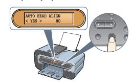
The pattern is printed. And Print Head is aligned automatically
