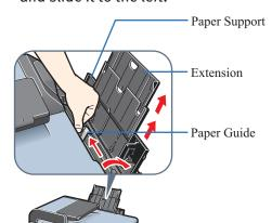
2 Load a few sheets of letter- or A4-size paper into the Auto Sheet Feeder, align the paper with the right side of the Cover Guide, then slide the Paper Guide toward the left edge of the paper.
