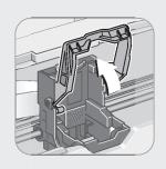
Slide the print head into the holder until it is securely seated.
