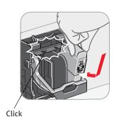
• Repeat the procedure for the color ink tank (BCI-24 Color), inserting it into the remaining slot. Close the front cover.
