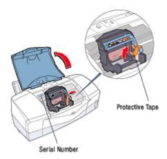
5. Write down the serial number located to the left of the printhead. You will need this later to register the product.
