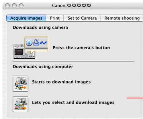
Camera Control Window with a Camera Connected
