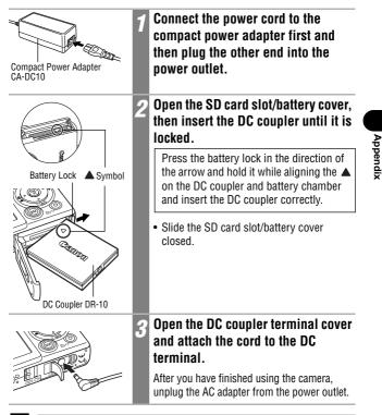
Use of an AC adapter kit other than ACK-DC10 (sold separately) may cause a malfunction in the camera or kit.
