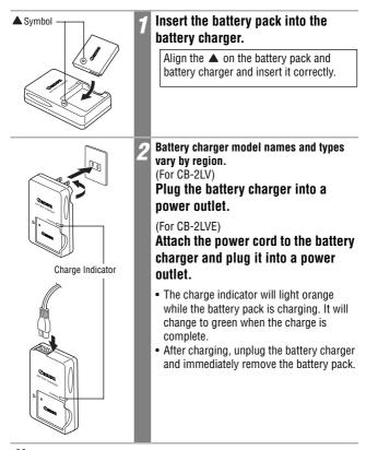
To protect the battery pack and prolong its life, do not charge it for longer than 24 hours continuously.
