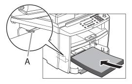
Adjust the paper guide rail to match the size of paper.
