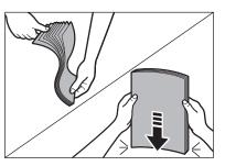
Load the paper into the paper cassette with the print side up. Make sure the paper stack sits below the small fin (A) on the side paper guide.
