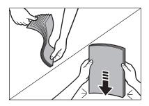
Load the paper into the paper feeding tray with the print side up. Make sure the paper stack sits below the hook (A) on the side paper guide.
