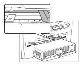
When setting paper, gently insert the paper into the multi-purpose tray with the print side up.
