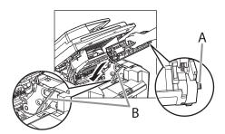
Push the toner cartridge to make sure it is 11 properly set in the machine.
