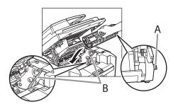
Push down the toner cartridge to make sure it is properly set in the machine.
