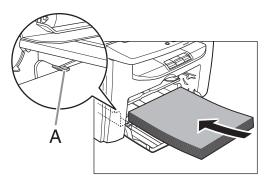
Adjust the paper guide rail to match the size of paper.
