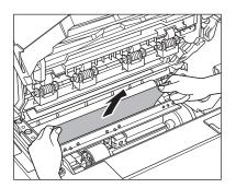
Hold both sides of the jammed paper and gently pull it out upward.
