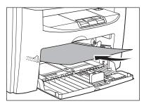
When setting an envelope, gently insert the envelope into the multi-purpose tray with the print side up and the right edge (i.e., closer to the stamp) first.
