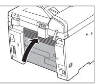
This operation is required only when <PAPER JAM/OPEN REAR COVER> appears on the display.
