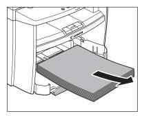
**15** Remove the paper cassette by lifting up the front-end of the paper cassette and pulling it forward.
