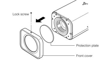
• When reattaching the protection plate, face the side with the cutout toward the lens.
