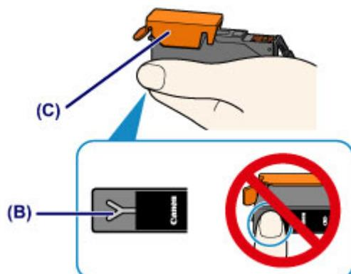
3. Lift up the tab on the orange protective cap (C) to remove it off GENTLY.
