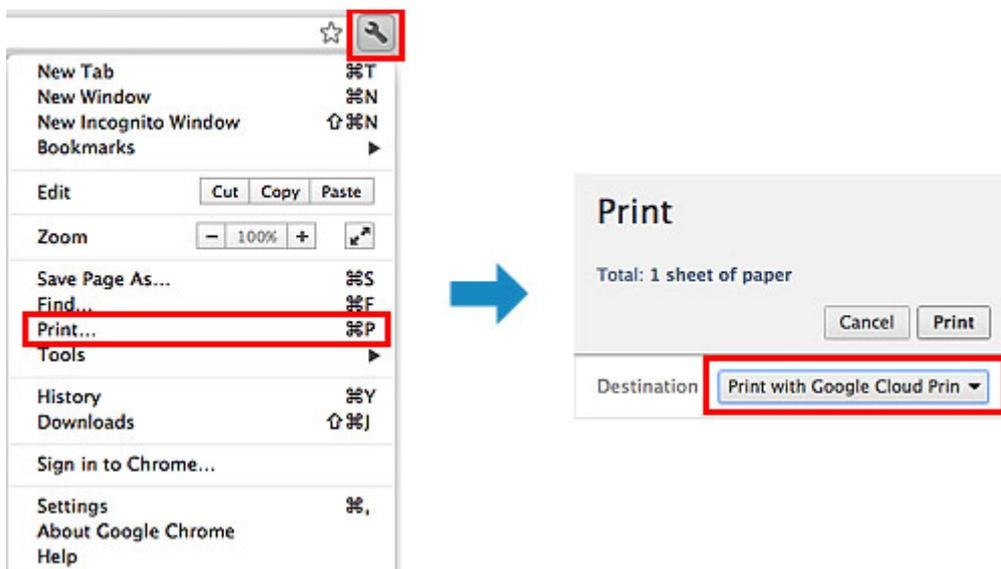
When the preparation for printing with Google Cloud Print is complete and when the machine is turned on, the machine receives the print data and prints it automatically.
