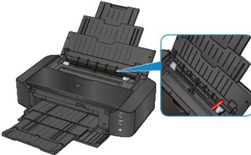
If there are any foreign objects in the rear tray, be sure to turn off the printer, unplug it from the power supply, then remove the foreign object.
