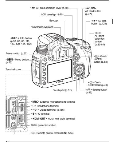
When connecting the interface cable to a digital terminal, also use the provided cable protector (p.27).
