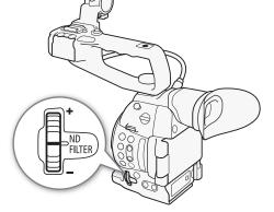
Turn the ND FILTER dial toward the + or - direction to select the desired ND filter setting.
