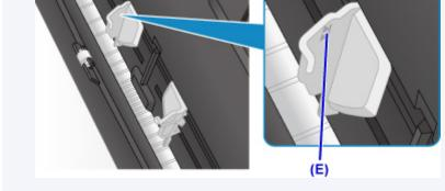
• Do not load envelopes higher than the load limit mark (E).
