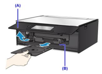
2. Place the printable disc with the printable surface facing up.
