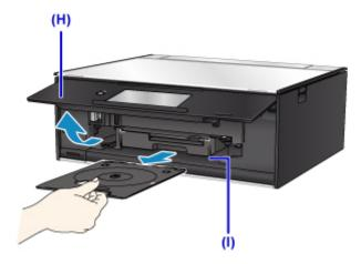
11. Place the printable disc with the printable surface facing up on the disc tray.
