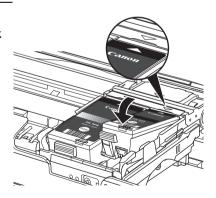
**5** Press on the Push mark on the ink tank until the ink tank snaps firmly into place.
