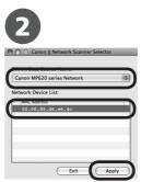
Select Canon MP620 series Network in TWAIN Data Source Name and the MAC address of the machine in **Network Device List**, then click **Apply** to use the machine as a scanner.
