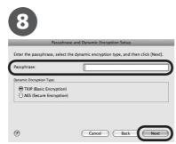
Enter your Passphrase (network password) and click Next. For the encryption method, the default setting (TKIP: Basic Encryption) should be used.
