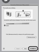
Confirm the measurement results, then click **Finish**. Ensure that is its displayed in Connection performance between the printer and the access point.
