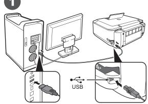
Connect one end of the USB cable to the computer and the other to the machine.
