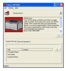
When a service call appears, cycle the power of the printer using the following procedure. This may clear the message.
