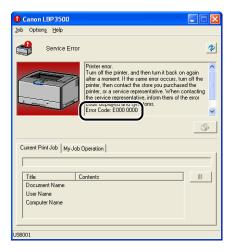
**3** Turn the printer and computer OFF ①, remove the USB cable ②, and then disconnect the power plug from the AC power outlet ③.
