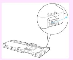
2 Remove the Ejection Guide.
