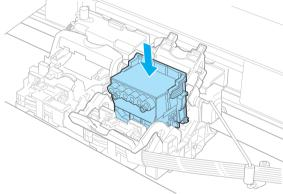
Pull the Printhead Fixer Cover down toward the front to lock the Printhead in place.
