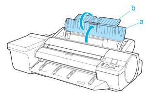
2 Slide the Width Guide (a) to align it with the mark for the size of paper you will load.
