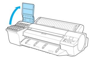
Lift the ink tank lock levers and remove all ink tanks.
