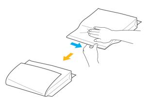
6 Put the used Maintenance Cartridge and packaging material in the box, just as the new Maintenance Cartridge was originally packaged, and store the used cartridge keeping it level.
