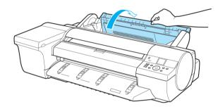
Holding the Roll Holder flange (a), load the Roll Holder shaft into the guide grooves (b) on both sides of the Roll Holder Slot. At this time, load the shaft so that the color of the Roll Holder shaft (c) matches the color of the guide groove.
