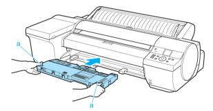
Hold the Ejection Guide on both sides by the near end. Aligning the Ejection Guide with the guides (a), insert it into the printer until it locks in place.
