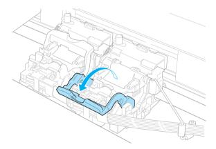
Pull up the Printhead Fixer Cover to open it completely.
