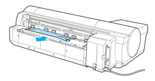
3 Attach the Roll Feed Unit to the printer. (See "Installing the Roll Feed Unit.") →User's Guide
