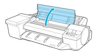
If the Printhead Fixer Cover or Printhead Fixer Lever is dirty, use a damp cloth that you have wrung out completely to wipe it clean.
