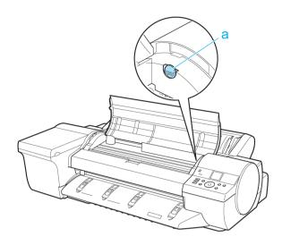
4 Using the back of the Cleaning Brush, move the first Switch to the side opposite ●.
