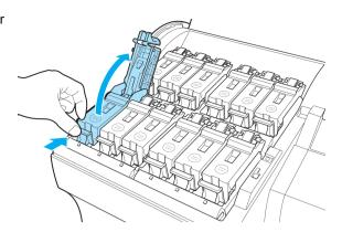
Hold the Ink Tank by the grips and remove it. Press the **OK** button.
