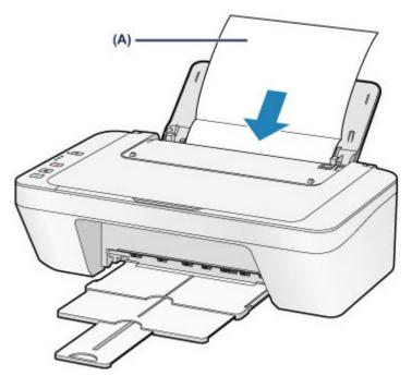
Load the paper (A) after unfolding it.
