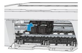
After confirming that the FINE cartridge is installed properly, close the cover.
