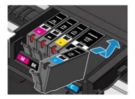
(2) Press on the top of the ink tank until the ink tank snaps firmly into place.
