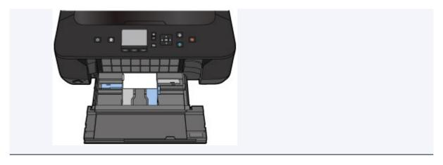
(6) Holding the right tab on the front tray, push the feeder back until the arrow (▶) on the front tray is aligned with the arrow (◄) on the machine.
