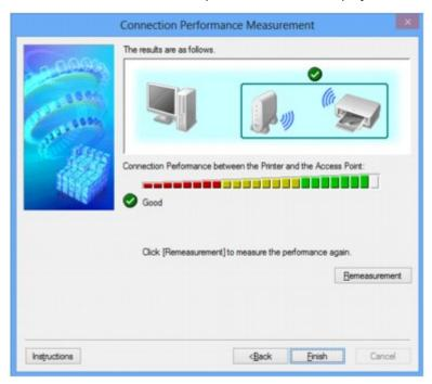
When so is displayed in Connection Performance between the Printer and the Access Point:, the printer can communicate with the access point. Otherwise, refer to displayed comments and the following to improve the status of communication link, and click **Remeasurement**.
