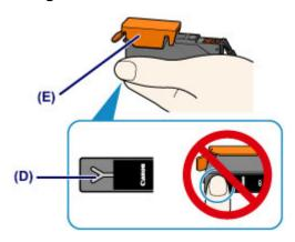
(3) Lift up the tab on the orange protective cap (E) to remove it off GENTLY.
