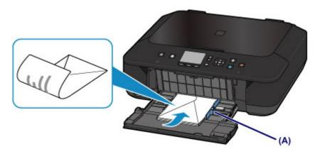
(5) Slide the right paper guide (A) to align the paper guides with both sides of the envelopes.
