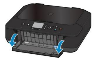
(2) Hold the right tab on the front tray to pull out the feeder until it stops.
