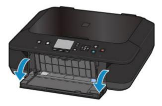
(2) Holding the right tab on the front tray, pull out the feeder until it stops.
