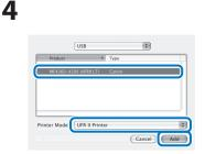
Select the machine (Canon Printer UFR II) from the list  $\rightarrow$  select [UFR II Printer] from [Printer Model]  $\rightarrow$  click [Add].
