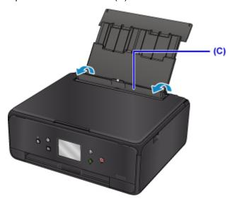
3. Slide the paper guides (D) to open them, and load the envelopes in the center of the rear tray WITH THE PRINT SIDE FACING UP.
