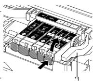
\*1 Do NOT touch the Print Head Lock Lever; remove only the ink tank.
