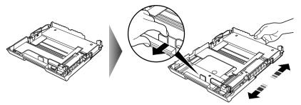
When loading  $5" \times 7"$  or smaller sized paper (nonstandard-size paper with less than 8 inches / 203 mm in length), do not extend the Cassette.
