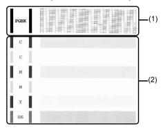
(1) If lines of this pattern are missing, the Black print head nozzle needs cleaning. Example: When lines are missing
