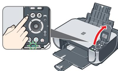
**4** Use the ▲ or ▼ button on the Operation Panel to select the language for the LCD, then press the OK button.
