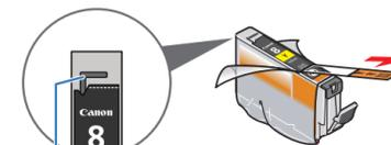
If the air hole is blocked with the remaining film, ink may leak out or may not eject properly.
