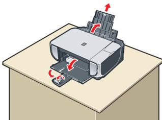
**2** Plug the power cord in the back of the machine and connect the other end to the wall outlet.
