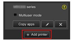
Select this to add printers to be used in the Canon Inkjet Cloud Printing Center. You need a Printer registration ID to add a printer.
