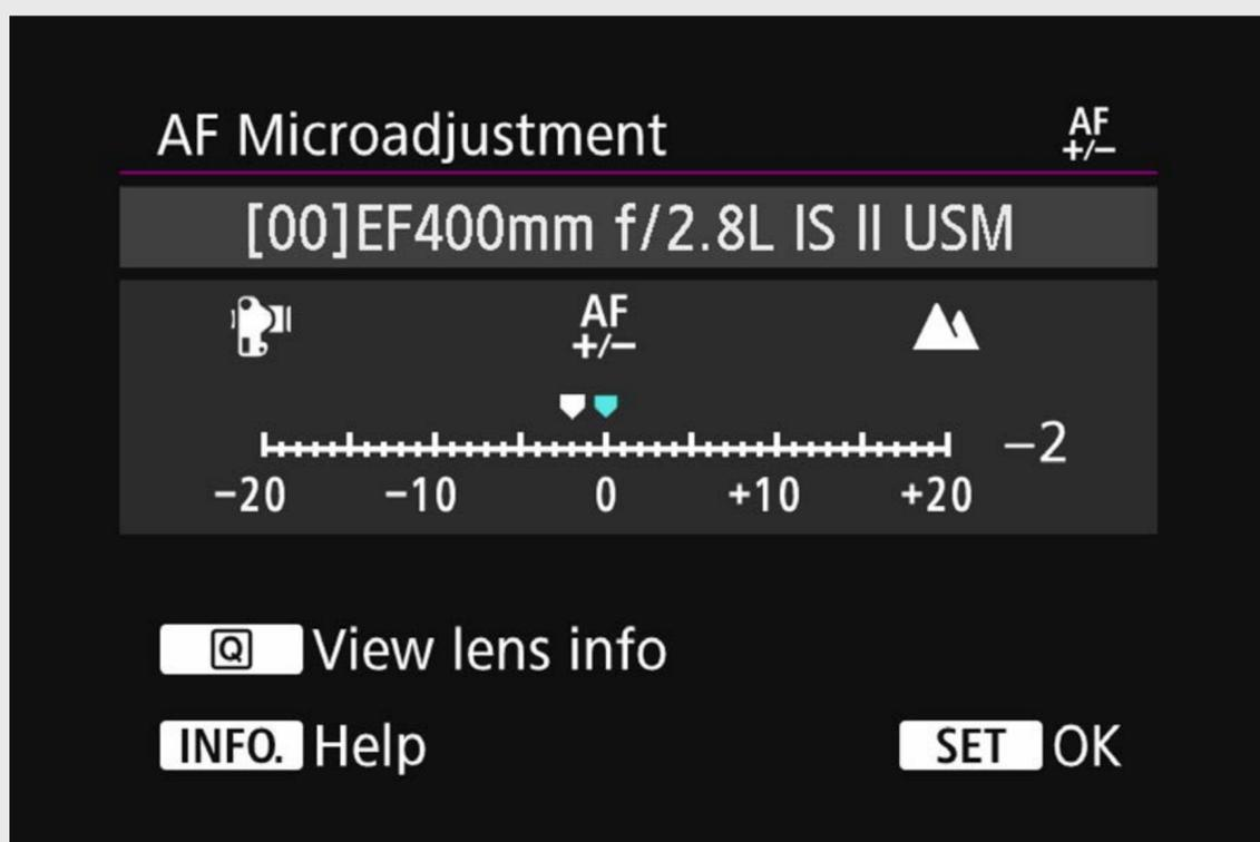
After entering an adjustment value, be sure to perform **test shooting** to **confirm** the result. After confirming it, if the adjustment value is insufficient, change it. Repeat this as necessary, and look for the suitable point of focus .
