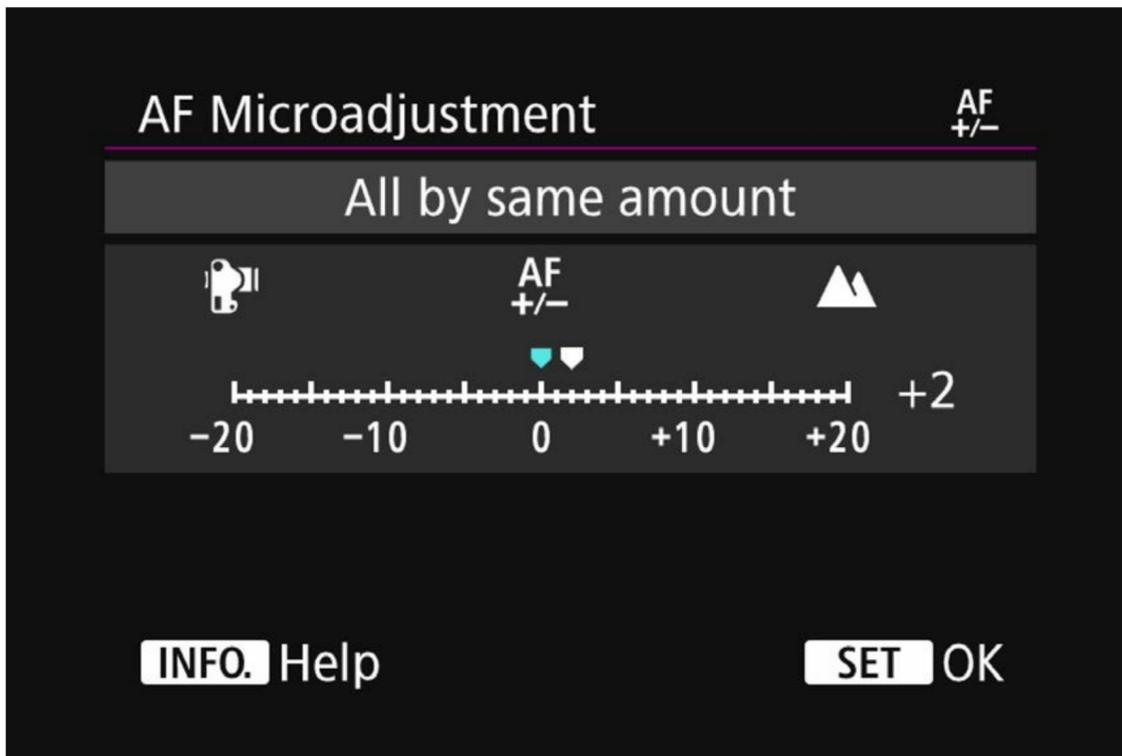
Turn the <
