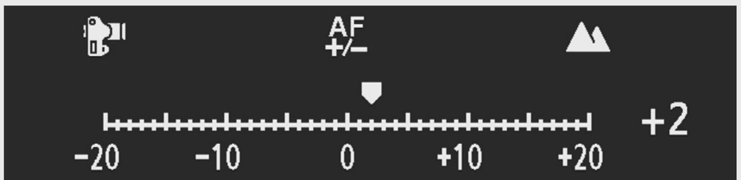
The adjustment quantity of one step will differ according to the maximum aperture of the lens being used. First, move two steps repeatedly making adjustments, shooting, and checking the results each time until the desired result is achieved.
