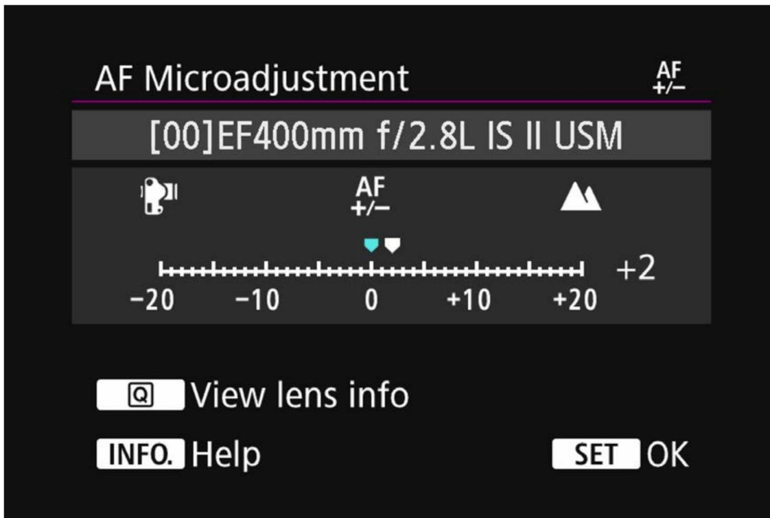
Turn the <
