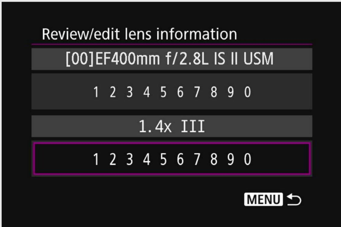
If [**Adjust by lens**] is selected and an extender is used, the adjustment will be registered for the lens and extender combination.
