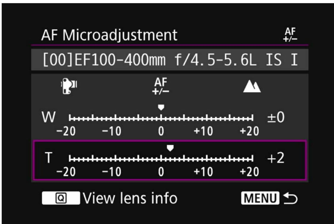
1. For a zoom lens, turn the <
