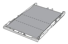
10. Mount the cassette cover, and then insert the cassette into the printer.
