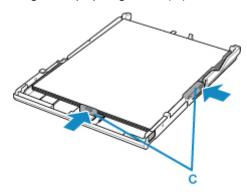
5. Mount the cassette cover, and then insert the cassette into the printer.
