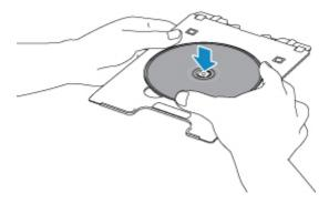
12. Insert the disc tray into the disc tray guide.
