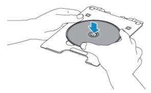
13. Insert the disc tray into the disc tray guide.
