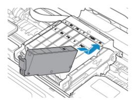
8. Press on the top of the ink tank until the ink tank snaps firmly into place.
