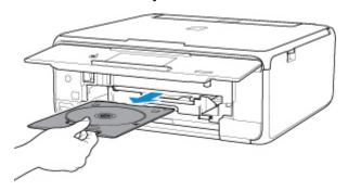
2. Remove the printable disc from the disc tray.
