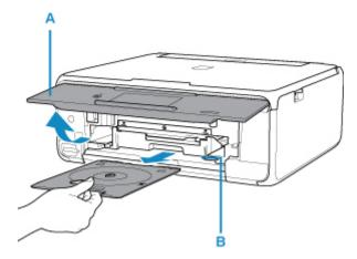
2. Place the printable disc with the printable surface facing up.
