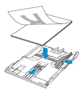
4. Align the paper guides (C) with the paper length and width.
