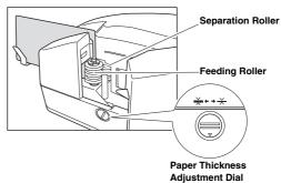
Slide the two sheets through between the feeding roller and the separation roller and stop at the position shown below.
