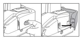
2 While lowering the open lever, open the reading unit.
