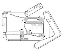
4 Use cotton swabs to clean the entire scanning glass. There are two scanning glass areas, one on each side. Use a cotton swab to wipe dirt from the entire surface of each.
