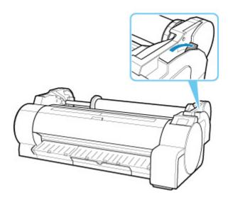
**3.** Fold an A4 sheet lengthwise four times and insert it through the gap of paper feed slot. Push scrap out toward platen.
