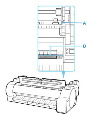
5. Pull the release lever forward and close the top cover.
