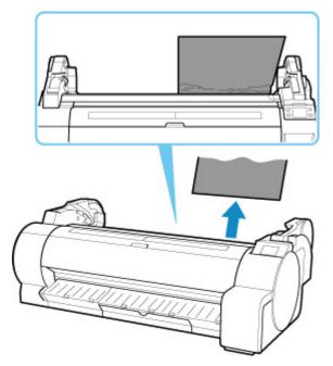
If the paper is jammed by the ejection guide
