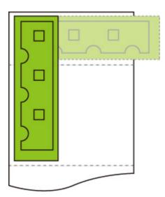
• Even if the image runs off the edge of the paper, it is rotated to expand the print range.
