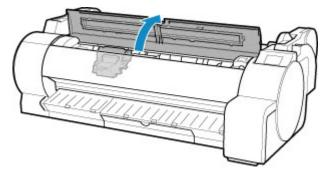
**5.** If the print head locking cover and print head lock lever are dirty, use a damp cloth that you have wrung out completely to wipe them clean.
