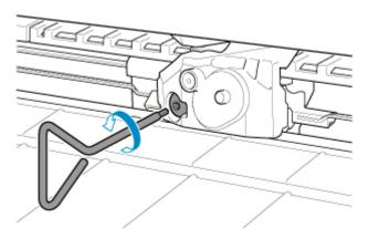
6. Remove cutter blade while holding A.
