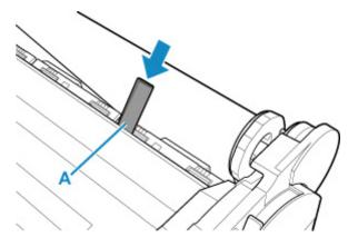
4. Remove scrap when it is pushed out onto platen.
