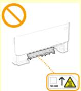
Do not carry the machine with any of the paper drawer or optional cassette feeding module installed. Otherwise, they may fall, resulting in injury.
