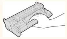
Do not touch the toner cartridge memory (a) or the electrical contacts (b). To avoid scratching the surface of the drum inside the machine or exposing it to light, do not open the drum protective shutter (a).
