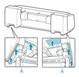
**2.** Remove tape and packaging material attached to the printer. Also open the top cover and remove stoppers and spacers inside the printer.
