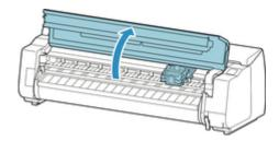
**7.** If the print head locking cover and print head lock lever are dirty, use a damp cloth that you have wrung out completely to wipe them clean.
