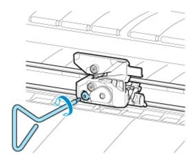
7. Remove cutter blade while holding D.
