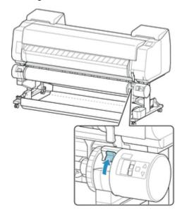
7. Hold roll holder by its flanges (A) and remove from roll holder slot.
