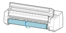
7. Hold Roll Holder by its flanges (A) and remove from roll holder slot.
