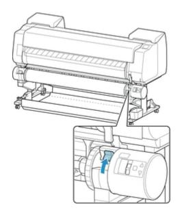
9. Hold roll holder by its flanges (A), and remove from roll unit.
