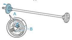
**3.** If taking up roll paper whose paper core has an inner diameter of 3 inches (76.2 mm), insert 3-Inch Paper Core Attachment in roll holder and holder stopper.
