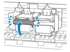
After confirming that the FINE cartridge is installed properly, close the cover.
