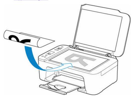
Align the corner of the original with the alignment mark  ${\bf \mbox{\sc 2}}$  .
