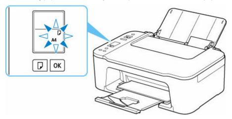
**7.** Press **Paper Select** button (H) to select a paper size according to the paper loaded on the rear tray and press **OK** button (I).
