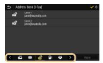
**4** Select the check box for the desired destination, and select <Apply>.
