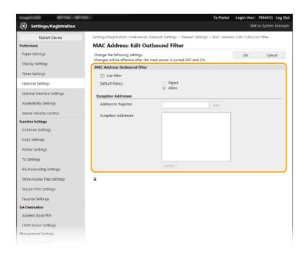
1 Select the [Use Filter] check box and click the [Reject] or [Allow] radio button for the [Default Policy].
