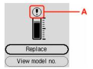
① The maintenance cartridge is almost full. Replace the maintenance cartridge as soon as possible.
