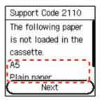
2. Select **Replace paper** with printer's **AV** buttons and press **OK** button.
