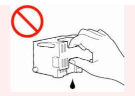
• Put the used one immediately into the plastic bag that came with the new maintenance cartridge and seal the bag by tying the opening tightly to prevent the ink from leaking.
