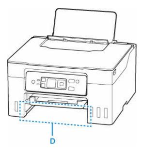
Removing Jammed Paper through Feed Slot of Cassette
