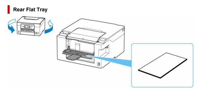
The rear flat tray is located at the rear of a printer.
