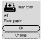
If the page size and the media type on the LCD matches the size of the paper loaded in the rear tray, select **OK**.
