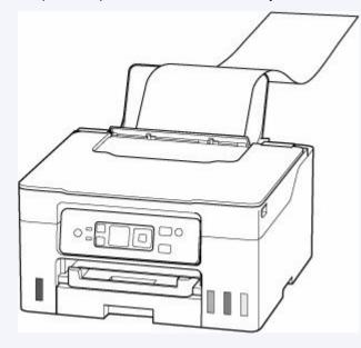
Move the right paper guide and adjust the guides to both edges of the paper stack.
