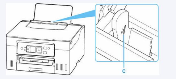
**6.** If page size and media type shown on LCD match size and type of envelopes loaded in rear tray, select **OK**.
