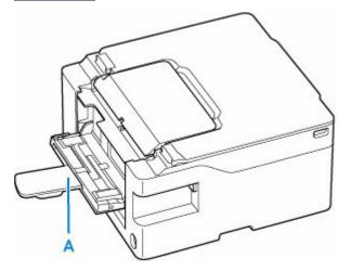
Removing Jammed Paper through Feed Slot of Rear Flat Tray
