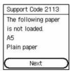
2. Select Print on set paper with printer's **AV** buttons and press **OK** button.
