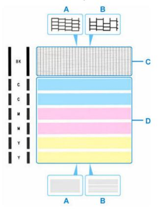
A: No missing lines/No horizontal streaksB: Lines are missing/Horizontal streaks are present
