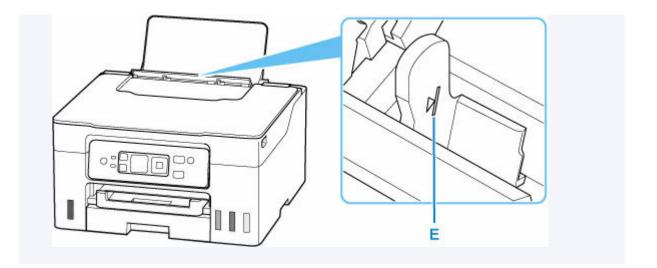
**6.** If page size and media type on LCD match size and type of paper loaded in rear tray, select **OK**.
