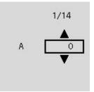
**9.** Examine the first print head position adjustment pattern, select the number of a pattern in which stripes are least noticeable in column A, and press the **OK** button.
