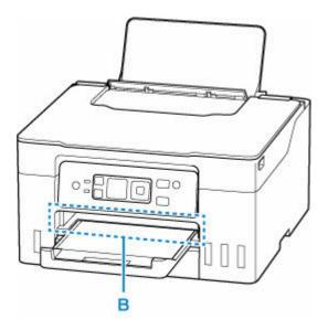
Removing Jammed Paper through Paper Output Slot
