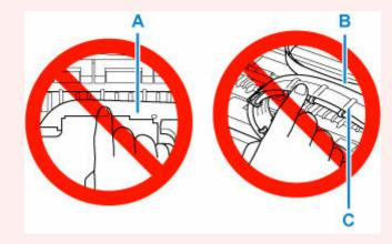
If you soil or scratch this part by touching it with paper or your hand, it could damage the printer.
